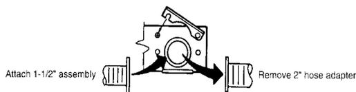
Remove 2" hose adaptor connection from machine. Attach AC1041 Accessory Hose 1 1/2" assembly with adaptor plate to vacuum lid inlet. Pull back female quick connect sleeve on the machine and insert male plug on the accessory solution hose. Attach upholstery tool or stair tool to the accessory hose.
