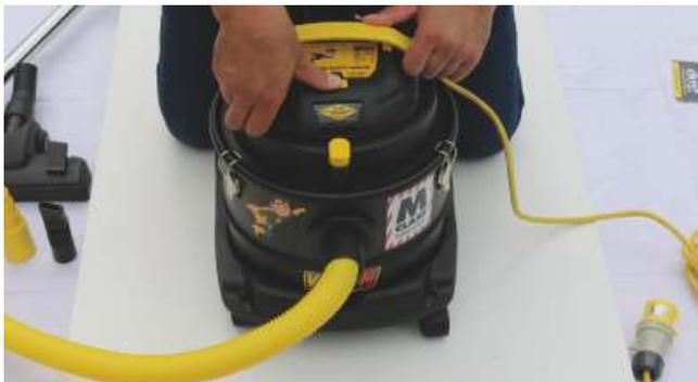
18 Plug in device then press switch to turn extraction on/off
