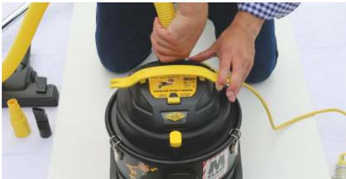
27 To use the blow feature, simply connect the hose to the exhaust port on top of the unit
