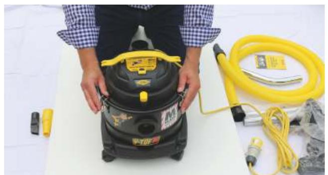
**12** Refit head and ensure all three clamps are fastened
