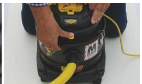
20 If monitor is red, press and hold Filter Shaker button for 10 seconds to clear filter (device/extraction must be on) If the monitor turns red only as and when you connect it to your power tool, ensure that the extraction passages of your tool are not blocked. If clear, it is OK to use. Just check the flow periodically by removing the extraction hose.
