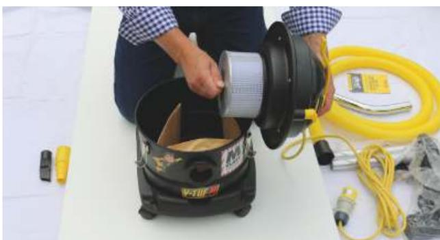
**11** Ensure the filter retainer screw is tight
